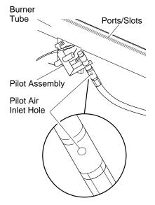
Figure 45 - Pilot Inlet Air Hole
